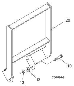
Figure 4. Grill Guard Installation
